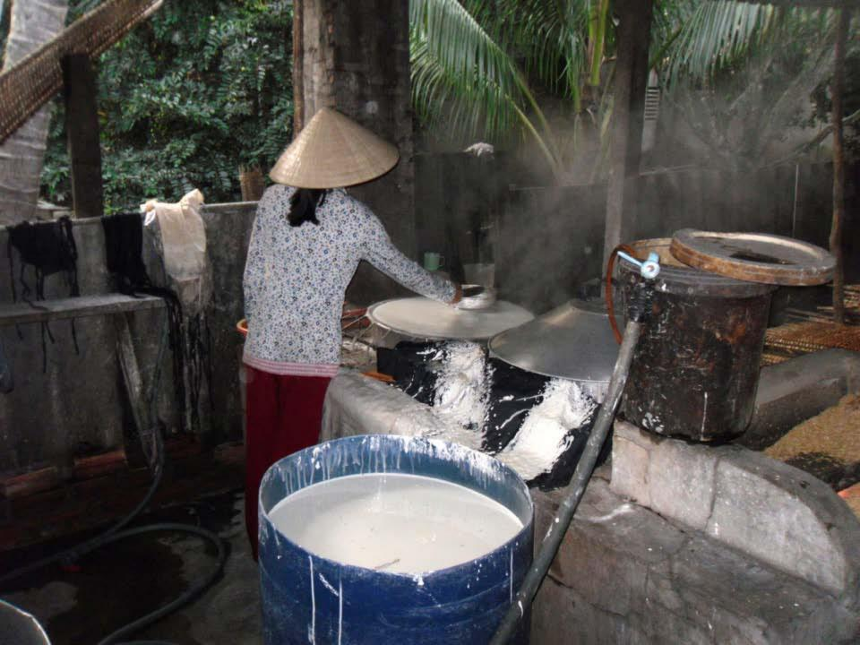
Rice husks are swept down from the trough to feed the furnace below. The conical lid steams the mix to give a milky translucence
